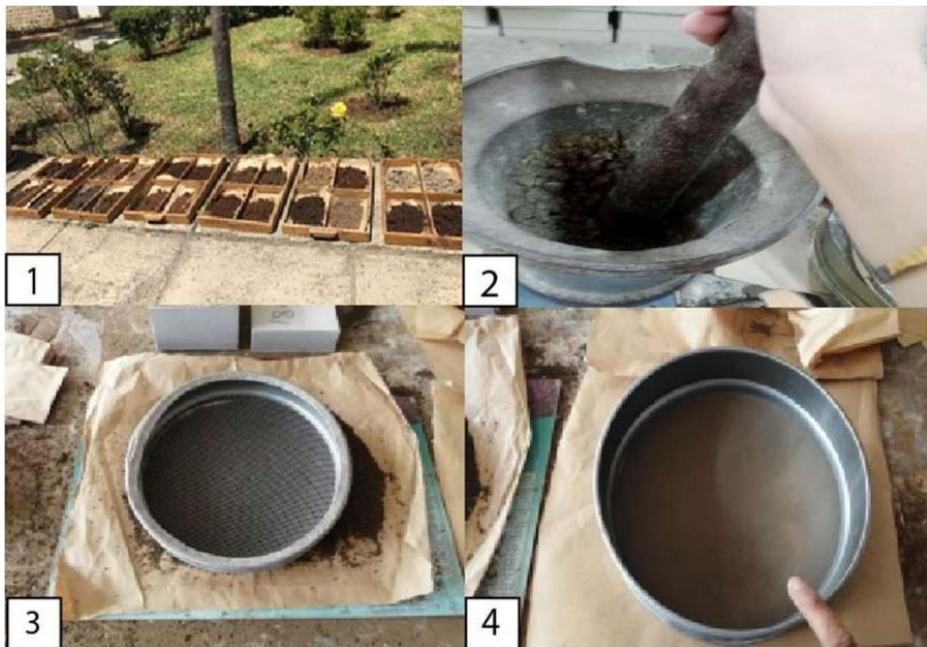
Fig 7: Soil sample preparation steps (1: Air drying, 2: Grinding, 3: 2mm sieving, 4: 0.2mm sieving).
